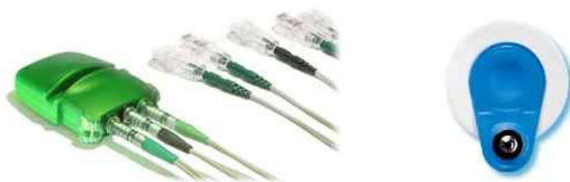
Figure 9: EMG module of the Biofeedback device 2000 x-pert by the company Schuhfried and one-way adhesive electrode Blue Sensor M by the company Ambu
