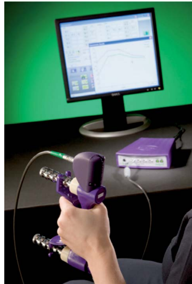
Fig. 22. Muscle strength assessment with the H500 dynamometer.
